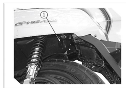
Emergency mechanical key (1)
