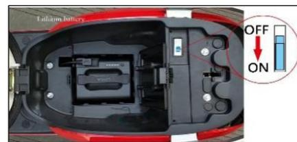
The "OFF" position of the main switch shown in the figure indicates that the power system of the vehicle is closed.
