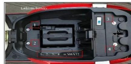
Open the Seat with the key, plug the battery cable inside the socket, connecting the battery with scooter.
