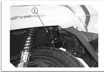
Emergency mechanical key (1)
